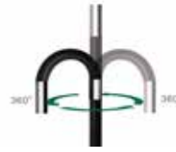
Robust articulation mechanism and probe bending for 360°
